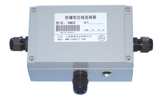
CM02 using the standard RS485 bus MODBUS-RTU protocol,easy access to PLC,DCS and other instruments or systems for monitoring 接线座 state quantities. The internal use of high-precision sensing core and related devices to ensure high reliability and excellent long-term stability, can be customized RS232,RS485,CAN,4-20mA,DC0~5V\10V,ZIGBEE,Lora,WIFI,GPRS and other output methods.
