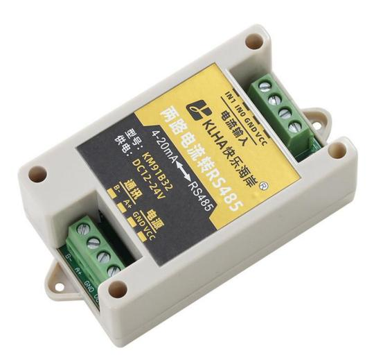
KM91B32 using the standard RS485 bus MODBUS-RTU protocol, easy access to PLC, DCS and other instruments or systems for monitoring 4-20mAcurrent,4-20mAcurrent state quantities. The internal use of high-precision sensing core and related devices to ensure high reliability and excellent long-term stability, can be customized RS232,RS485,CAN,4-20mA,DC0~5V\10V,ZIGBEE,Lora,WIFI,GPRS and other output methods.
