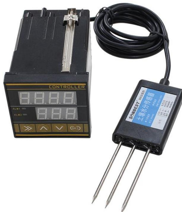
Soil moisture temperature controller, also known as soil temperature and humidity controller, soil temperature and humidity controller, is mainly composed of two parts: controller instrument, soil moisture sensor. The controller has high reliability and stability, It meets the needs of users in many aspects. The
