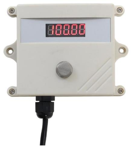
SD2130V-NH3 using the standard DC0 ~ 10V voltage output signal,easy access to PLC, DCS and other instruments or systems for monitoring ammonia state quantities. The internal use of high-precision sensing core and related devices to ensure high reliability and excellent long-term stability,can be customized RS232,RS485,CAN,4-20mA,DC0~5V\10V,ZIGBEE,Lora,WIFI,GPRS and other output methods.
