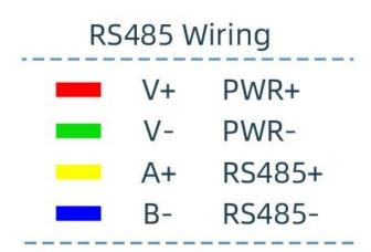
※Note: Connect the positive and negative poles of the power supply first, and then connect the signal wire
