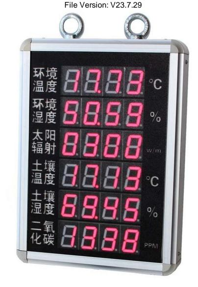
SD8603B using the standard RS485 bus MODBUS-RTU protocol, easy access to PLC, DCS and other instruments or systems for monitoring temperature, humidity, carbon dioxide, soil Moisture, soil temperature, Radioactivity state quantities. The internal use of high-precision sensing core and related
