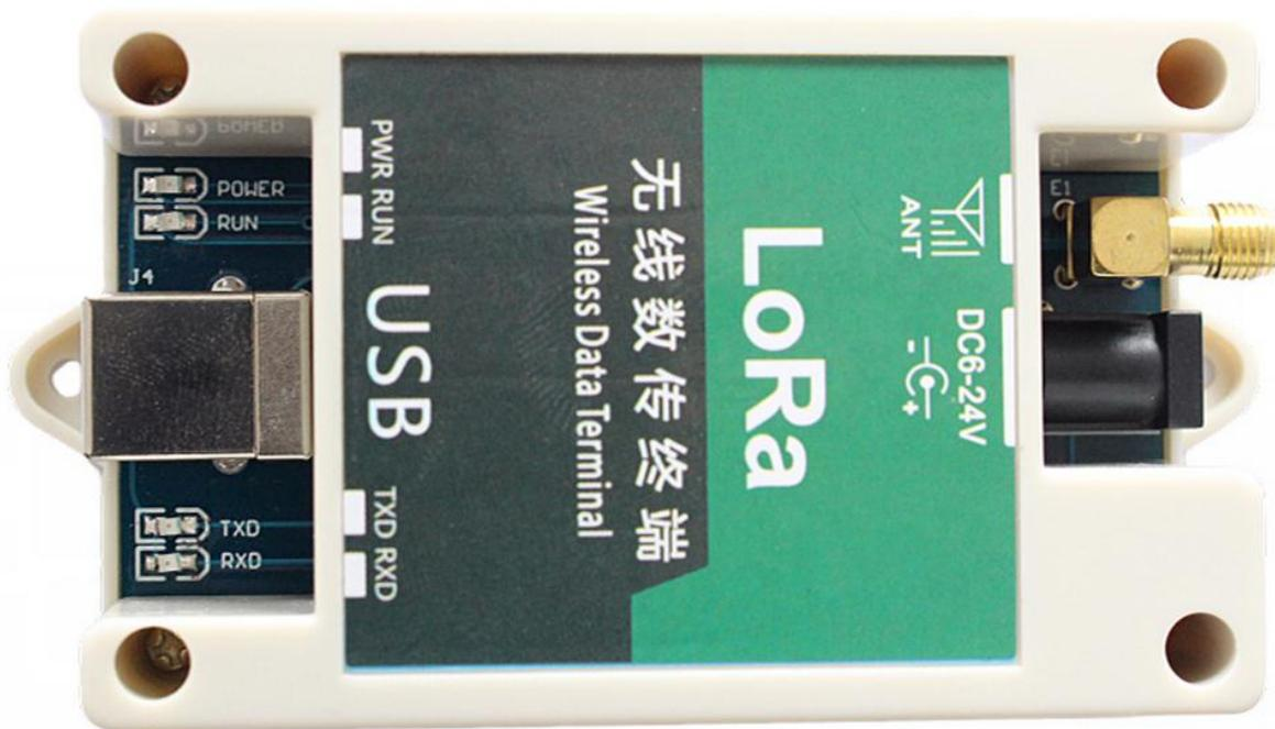
SL9192U using the standard USB, easy access to PLC, DCS and other instruments or systems for monitoring LORA state quantities. The internal use of high-precision sensing core and related devices to
