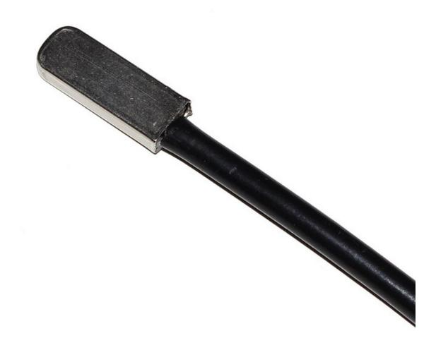
Suobo SLST2 series PT100 sensor platinum resistance is made of platinum wire with a purity of 99.9995%. It has stable performance,good repeatability,high precision and good linearity in a certain temperature range. It is an internationally recognized mature product. The international temperature
