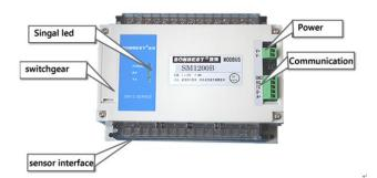
As shown in the above, the equipment by the power supply interface, RS485 interface, sensor wiring, calibration status indicator lights, button and pull code switch.
