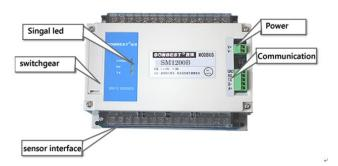
As shown in the above, the equipment by the power supply interface, RS485 interface, sensor wiring, calibration status indicator lights, button and pull code switch.
