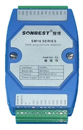
SM1603B using the standard RS485 bus MODBUS-RTU protocol, easy access to PLC, DCS and other instruments or systems for monitoring temperature state quantities. The internal use of high-precision sensing core and related devices to ensure high reliability and excellent long-term stability, can be customized RS232,RS485,CAN,4-20mA,DC0~5V\10V,ZIGBEE,Lora,WIFI,GPRS and other output methods.
