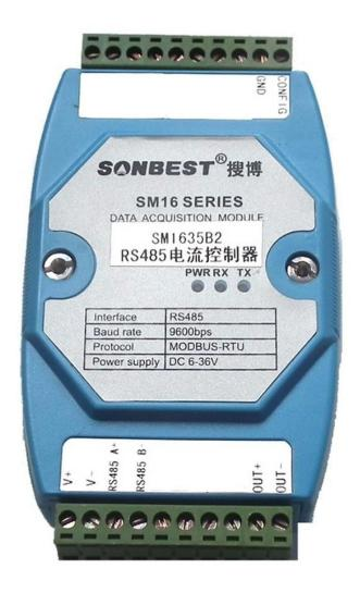
SM1635B2 using the standard RS485 bus MODBUS-RTU protocol, easy access to PLC, DCS and other instruments or systems for monitoring 4-20MAcurrent state quantities. The internal use of high-precision sensing core and related devices to ensure high reliability and excellent long-term stability, can be customized RS232, RS485, CAN, 4-20mA, DC0~5V\10V, ZIGBEE, Lora, WIFI, GPRS and other output methods.
