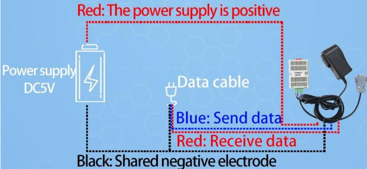
Din rail temperature sensor can be widely used in animal breeding, file management, food storage, greenhouses, drug storage, tobacco industry, industrial control industry and other indoor temperature and humidity measurement fields
