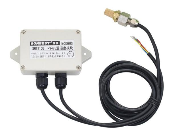
SM1910B using the standard RS485 bus MODBUS-RTU protocol, easy access to PLC, DCS and other instruments or systems for monitoring temperature, humidity state quantities. The internal use of high-precision sensing core and related devices to ensure high reliability and excellent long-term stability, can be customized RS232, RS485, CAN, 4-20mA, DC0~5V\10V, ZIGBEE, Lora, WIFI, GPRS and other output methods.
