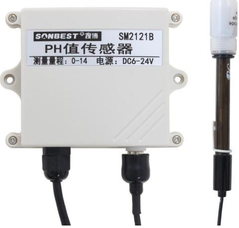
SM2121B using the standard RS485 bus MODBUS-RTU protocol, easy access to PLC, DCS and other instruments or systems for monitoring pH state quantities. The internal use of high-precision sensing core and related devices to ensure high reliability and excellent long-term stability, can be customized RS232,RS485,CAN,4-20mA,DC0~5V\10V,ZIGBEE,Lora,WIFI,GPRS and other output methods.
