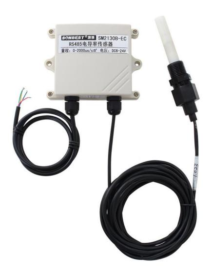
SM2130B-EC using the standard RS485 bus MODBUS-RTU protocol, easy access to PLC, DCS and other instruments or systems for monitoring conductivity state quantities. The internal use of high-precision sensing core and related devices to ensure high reliability and excellent long-term stability, can be customized RS232,RS485,CAN,4-20mA,DC0~5V\10V,ZIGBEE,Lora,WIFI,GPRS and other output methods.
