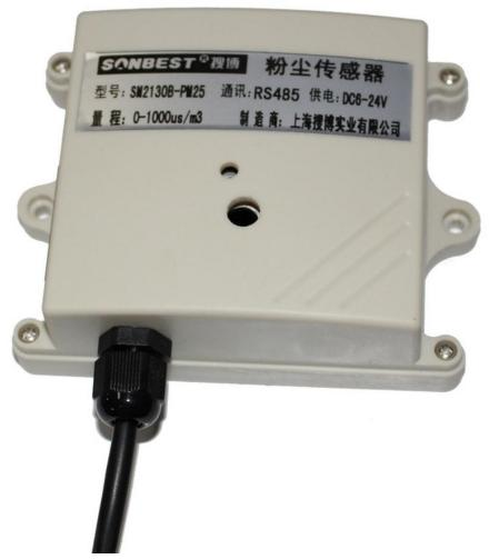
SM2130B-PM25 using the standard RS485 bus MODBUS-RTU protocol, easy access to PLC, DCS and other instruments or systems for monitoring PM2.5 state quantities. The internal use of high-precision sensing core and related devices to ensure high reliability and excellent long-term stability, can be customized RS232,RS485,CAN,4-20mA,DC0~5V\10V,ZIGBEE,Lora,WIFI,GPRS and other output methods.
