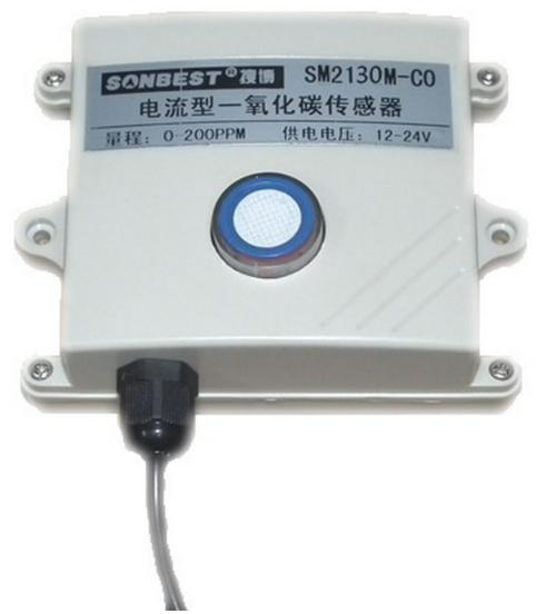
SM2130M-CO using the standard DC4-20mA current output signal, easy access to PLC, DCS and other instruments or systems for monitoring carbon monoxide state quantities. The internal use of high-precision sensing core and related devices to ensure high reliability and excellent long-term stability, can be customized RS232,RS485,CAN,4-20mA,DC0~5V\10V,ZIGBEE,Lora,WIFI,GPRS and other output methods.
