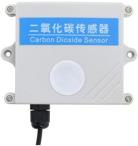
SM2130M-CO2 using the standard DC4-20mA current output signal, easy access to PLC, DCS and other instruments or systems for monitoring carbon dioxide state quantities. The internal use of high-precision sensing core and related devices to ensure high reliability and excellent long-term stability, can be customized RS232, RS485, CAN, 4-20mA, DC0~5V\10V, ZIGBEE, Lora, WIFI, GPRS and other output methods.
