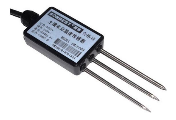
SM2802B using the standard RS485 bus MODBUS-RTU protocol, easy access to PLC, DCS and other instruments or systems for monitoring 24%soil Moisture, soil temperature state quantities. The internal use of high-precision sensing core and related devices to ensure high reliability and excellent long-term stability, can be customized RS232, RS485, CAN, 4-20mA, DC0~5V\10V, ZIGBEE, Lora, WIFI, GPRS and other output methods.
