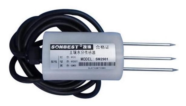
SM2901V2 using the standard ,easy access to PLC, DCS and other instruments or systems for monitoring 24%soil Moisture state quantities. The internal use of high-precision sensing core and related devices to ensure high reliability and excellent long-term stability,can be customized RS232,RS485,CAN,4-20mA,DC0~5V\10V,ZIGBEE,Lora,WIFI,GPRS and other output methods.
