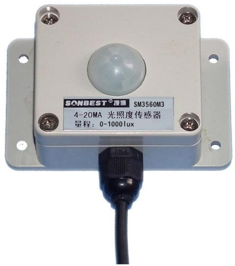
SM3560M3 using the standard ,easy access to PLC, DCS and other instruments or systems for monitoring Illuminance state quantities. The internal use of high-precision sensing core and related devices to ensure high reliability and excellent long-term stability, can be customized
