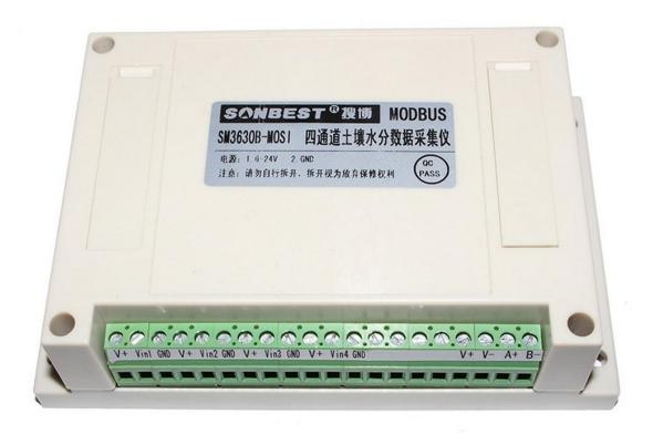
SM3630B-MOSI using the standard RS485 bus MODBUS-RTU protocol, easy access to PLC, DCS and other instruments or systems for monitoring soil Moisture state quantities. The internal use of high-precision sensing core and related devices to ensure high reliability and excellent long-term stability, can be customized RS232, RS485, CAN, 4-20mA, DC0~5V\10V, ZIGBEE, Lora, WIFI, GPRS and other output methods.
