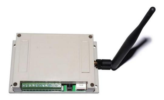
SM3650T using the standard TCP/IP Network Interface, easy access to PLC, DCS and other instruments or systems for monitoring state quantities. The internal use of high-precision sensing core and related devices to ensure high reliability and excellent long-term stability, can be customized RS232,RS485,CAN,4-20mA,DC0~5V\10V,ZIGBEE,Lora,WIFI,GPRS and other output methods.
