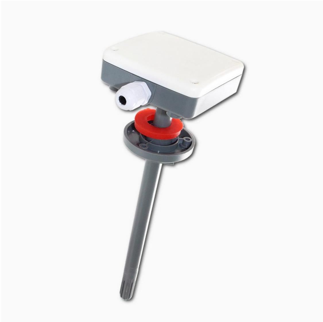
SM3710M2 using the standard ,easy access to PLC , DCS and other instruments or systems for monitoring temperature,humidity state quantities.The internal use of high-precision sensing core and related devices to ensure high reliability and excellent long-term stability,can be customized RS232,RS485,CAN,4-20mA,DC0~5V\10V,ZIGBEE,Lora,WIFI,GPRS and other output methods.
