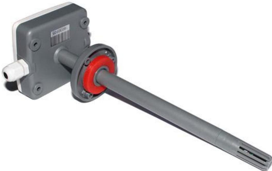
SM3710V2 using the standard DC0 ~ 10V voltage output signal,easy access to PLC , DCS and other instruments or systems for monitoring temperature,humidity state quantities.The internal use of high-precision sensing core and related devices to ensure high reliability and excellent long-term stability,can be customized RS232,RS485,CAN,4-20mA,DC0~5V10V,ZIGBEE,Lora,WIFI,GPRS and other output methods.
