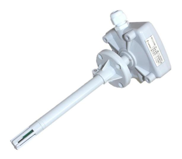
SM3810B using the standard RS485 bus MODBUS-RTU protocol, easy access to PLC, DCS and other instruments or systems for monitoring temperature, humidity state quantities. The internal use of high-precision sensing core and related devices to ensure high reliability and excellent long-term stability, can be customized RS232, RS485, CAN, 4-20mA, DC0~5V\10V, ZIGBEE, Lora, WIFI, GPRS and other output methods.
