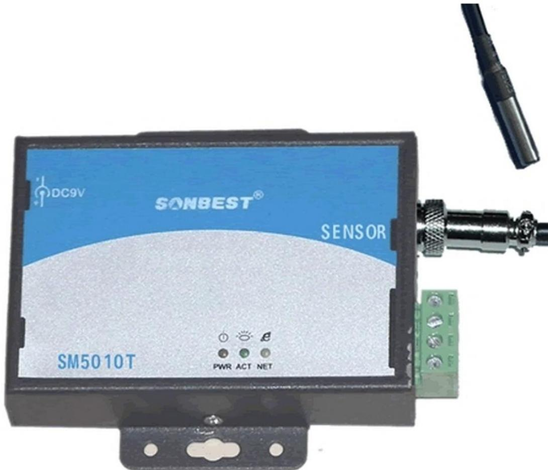
SM500T using the standard TCP/IP Network Interface, easy access to PLC, DCS and other instruments or systems for monitoring temperature state quantities. The internal use of high-precision sensing core and related devices to ensure high reliability and excellent long-term stability, can be customized RS232, RS485, CAN, 4-20mA, DC0~5V\10V, ZIGBEE, Lora, WIFI, GPRS and other output methods.
