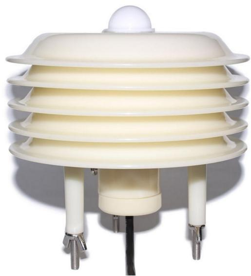
SM639XB using the standard RS485 bus MODBUS-RTU protocol, easy access to PLC, DCS and other instruments or systems for monitoring conductivity, temperature, humidity, Illuminance, atmospheric pressure state quantities. The internal use of high-precision sensing core and related devices to ensure high reliability and excellent long-term stability, can be customized
