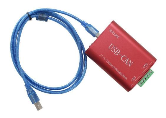
SU8190C using the standard USB, easy access to PLC, DCS and other instruments or systems for monitoring CAN2 state quantities. The internal use of high-precision sensing core and related devices to ensure high reliability and excellent long-term stability, can be customized RS232,RS485,CAN,4-20mA,DC0~5V\10V,ZIGBEE,Lora,WIFI,GPRS and other output methods.
