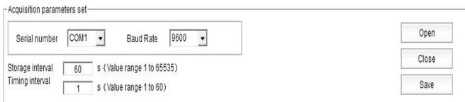
**【Serial number】** here with the actual access serial port number, if the desktop, usually COM1 or COM2, or USB converter mapped into a serial port, the general COM3-16, can access the computer hardware information in the query .
