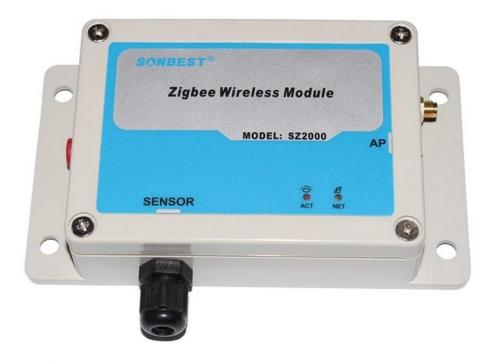
SZ2000 using the standard ZIGBEE Wireless Communication Interface, easy access to PLC, DCS and other instruments or systems for monitoring RS485 state quantities. The internal use of high-precision sensing core and related devices to ensure high reliability and excellent long-term stability, can be customized RS232, RS485, CAN, 4-20 mA, DC0~5V\10V, ZIGBEE, Lora, WIFI, GPRS and other output methods.
