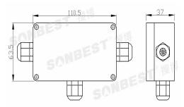
1-4 Branch CM02 wiring outline and box PCB circuit diagram as shown below:
