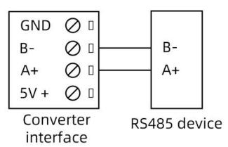
Note: When the power supply of the user equipment is DC5V, the converter can directly supply power to the user equipment, GND is the negative pole of the power supply, and 5V is the positive pole of the power supply. It can only supply power to devices with a power supply of 5V
