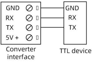
Note: When the power supply of the user equipment is DC5V, the converter can directly supply power to the user equipment, GND is the negative pole of the power supply, and 5V is the positive pole of the power supply. You can only supply power to devices with a power supply of 5V.
