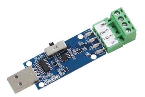
HD811 using the standard USB,easy access to PLC, DCS and other instruments or systems for monitoring RS485,TTL state quantities.The internal use of high-precision sensing core and related devices to ensure high reliability and excellent long-term stability,can be customized
