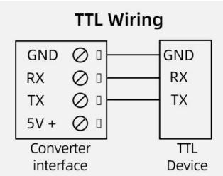
Note: The switch goes to TTL, when the user equipment power supply is DC5V, the converter can directly supply power to the user equipment
