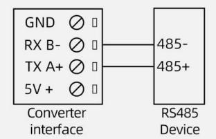
Note: The switch goes to 485. When the power supply of the user equipment is DC5V, the converter can directly supply power to the user equipment, GND is the negative power supply, and 5V is the positive power supply. Can only supply power to devices with 5V power supply
