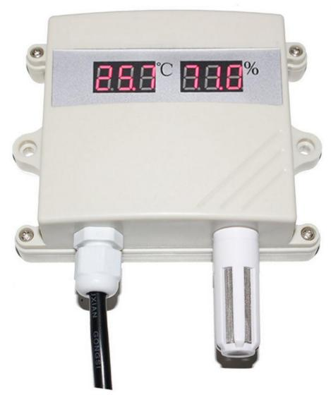
KD2110V using the standard DC0 ~ 5V voltage output signal, easy access to PLC, DCS and other instruments or systems for monitoring temperature, humidity state quantities. The internal use of high-precision sensing core and related devices to ensure high reliability and excellent long-term stability, can be customized RS232, RS485, CAN, 4-20 mA, DC0~5V\10V, ZIGBEE, Lora, WIFI, GPRS and other output methods.
