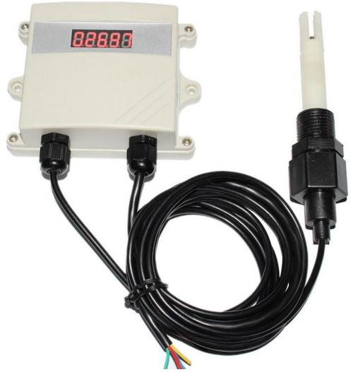
KD2130B-EC using the standard RS485 bus MODBUS-RTU protocol,easy access to PLC, DCS and other instruments or systems for monitoring conductivity state quantities. The internal use of high-precision sensing core and related devices to ensure high reliability and excellent long-term stability, can be customized RS232,RS485,CAN,4-20mA,DC0~5V\10V,ZIGBEE,Lora,WIFI,GPRS and other output methods.
