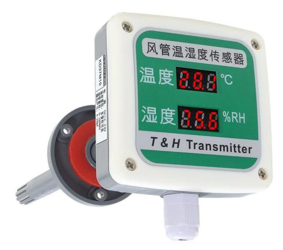
KD37B10 using the standard ,easy access to PLC, DCS and other instruments or systems for monitoring temperature,humidity state quantities. The internal use of high -precision sensing core and related devices to ensure high reliability and excellent long-term stability,can be customized RS232,RS485,CAN,4-20mA,DC0~5V\10V,ZIGBEE,Lora,WIFI,GPRS and other output methods.
