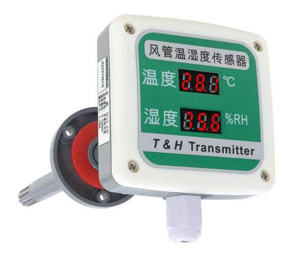
KD37M10 using the standard ,easy access to PLC. DCS and other instruments or systems for monitoring temperature, humidity state quantities. The internal use of high-precision sensing core and related devices to ensure high reliability and excellent long-term stability, can be customized RS232,RS485,CAN,4-20mA,DC0~5V\10V,ZIGBEE,Lora,WIFI,GPRS and other output methods.
