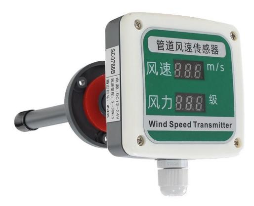
KD37M88 using the standard DC4-20mA current output signal, easy access to PLC, DCS and other instruments or systems for monitoring wind speed state quantities. The internal use of high-precision sensing core and related devices to ensure high reliability and excellent long-term stability, can be customized RS232, RS485, CAN, 4-20mA, DC0~5V\10V, ZIGBEE, Lora, WIFI, GPRS and other output methods.
