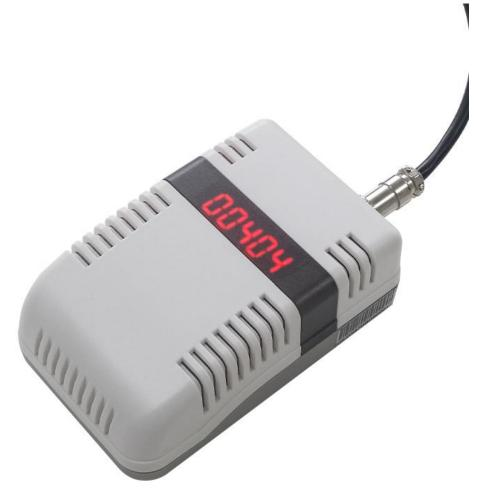
KD58B70 using the standard ,easy access to PLC. DCS and other instruments or systems for monitoring carbon dioxide state quantities. The internal use of high-precision sensing core and related devices to ensure high reliability and excellent long-term stability, can be customized RS232,RS485,CAN,4-20mA,DC0~5V\10V,ZIGBEE,Lora,WIFI,GPRS and other output methods.
