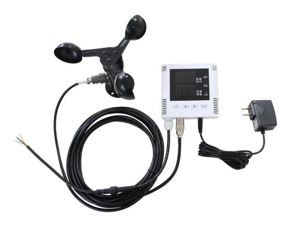
KD67B86 using the standard RS485 bus MODBUS-RTU protocol, easy access to PLC, DCS and other instruments or systems for monitoring wind speed state quantities. The internal use of high-precision sensing core and related devices to ensure high reliability and excellent long-term stability, can be customized RS232, RS485, CAN, 4-20mA, DC0~5V\10V, ZIGBEE, Lora, WIFI, GPRS and other output methods.
