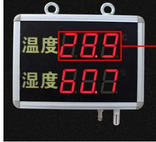
Remote real-time monitoring of the temperature, to prevent the temperature from being exceeded and lower than the lower limit, the negative number of the temperature does not display 1 decimal place
