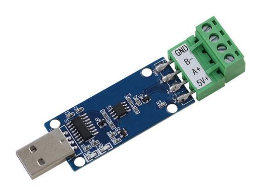
KL815 using the standard USB, easy access to PLC, DCS and other instruments or systems for monitoring RS485,TTL state quantities. The internal use of high-precision sensing core and related devices to ensure high reliability and excellent long-term stability, can be customized
