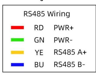
※Note: When wiring, connect the positive and negative poles of the power supply first, and then connect the signal wire
