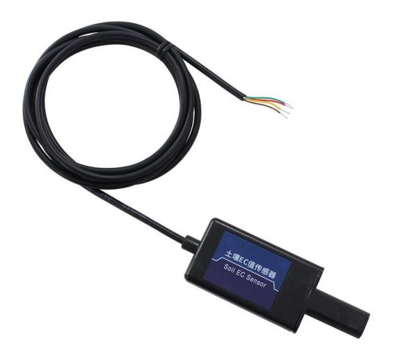
KM31B05 using the standard ,easy access to PLC, DCS and other instruments or systems for monitoring  $\pm \bar{\mu}$  conductivity state quantities. The internal use of high-precision sensing core and related devices to ensure high reliability and excellent long-term stability, can be customized RS232,RS485,CAN,4-20mA,DC0~5V\10V,ZIGBEE,Lora,WIFI,GPRS and other output methods.
