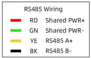
XNote: When wiring, connect the positive and negative poles of the power supply first, and then connect the signal wire
