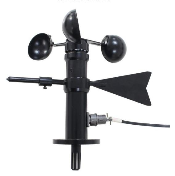
KM53B98 using the standard RS485 bus MODBUS-RTU protocol, easy access to PLC, DCS and other instruments or systems for monitoring wind speed, conductivity, temperature, humidity state quantities. The internal use of high-precision sensing core and related devices to ensure high reliability and
