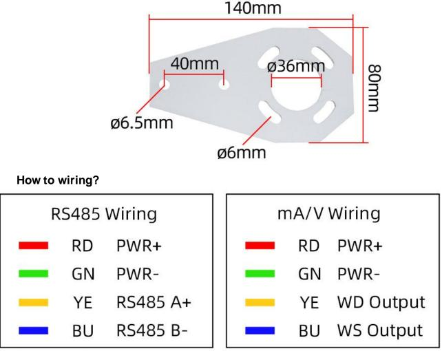
XNote: When wiring, connect the positive and negative poles of the power supply first, and then connect the signal wire
