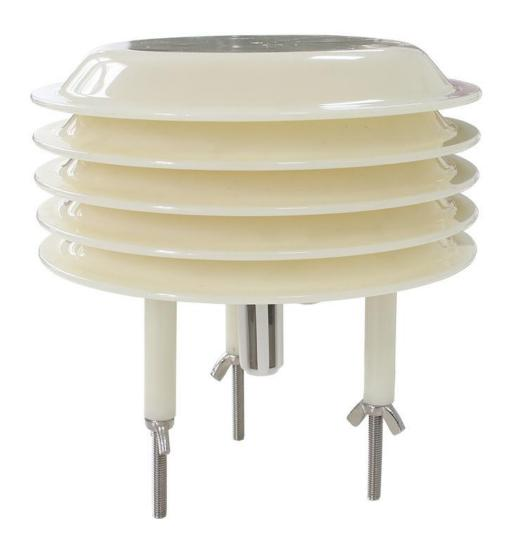
KM63B13 using the standard RS485 bus MODBUS-RTU protocol, easy access to PLC, DCS and other instruments or systems for monitoring temperature, humidity state quantities. The internal use of high-precision sensing core and related devices to ensure high reliability and excellent long-term stability, can be customized RS232, RS485, CAN, 4-20mA, DC0~5V\10V, ZIGBEE, Lora, WIFI, GPRS and other output methods.
